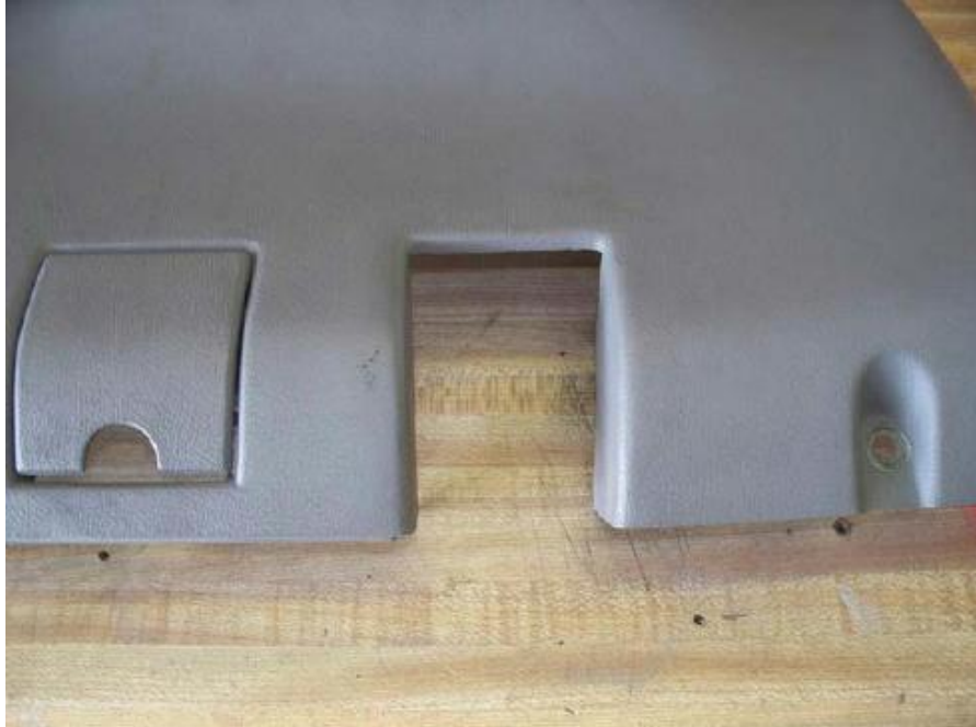
Photo 1: Hood Latch Section Removed.
