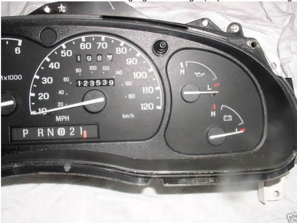
This section will just pull straight out with no screws once the lens is removed.
