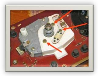
\*Some speedometers have these additional electronic connections. If yours does, then remove the **smaller slotted screws** shown.
