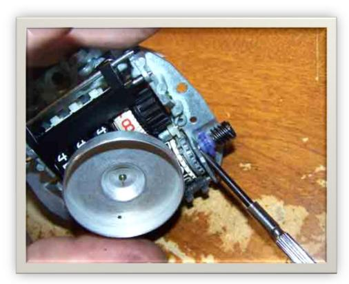
REMOVING THE OUTSIDE GEARS: If you need to remove the outside gears, **gently** pry them with a small flat screwdriver (see photo). I don't know yet if it matters, but for now **pay close attention to which direction they face**, so you can put them back on the same way.
