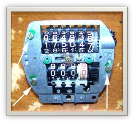
\*Here's the naked speedometer after removing the faceplate.
