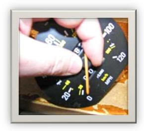
\*Now, after gently lifting the needle over the stop pin, grip the center plastic hub of the Speedo needle and turn it counter-clockwise (toward the "MPH"). **Be careful not to put pressure on**
