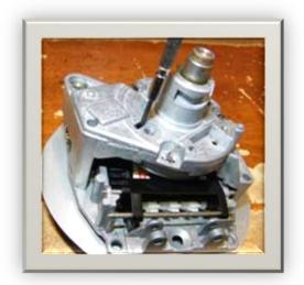
Insert a small slotted screwdriver (like the one shown) into one of the holes. This will lock the speed cup and mechanism inside the speedometer so the needle shaft cannot move.
