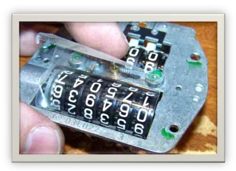
I found a way. The shaft needs to be pulled out just enough to release this metal gear. The last thing I wanted to see was all those little number wheels falling out, or even moving in the slightest amount. So I applied a piece of **packing tape** across the wheels (see photo) to keep them snugly together. No moving equals much, much better.
