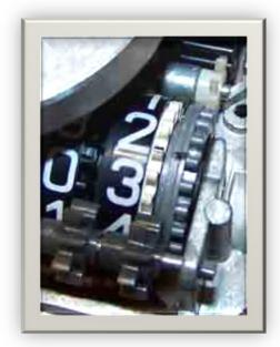
\*Then I used a felt marker and marked both the gray metal gear and the white plastic one next to it. I wanted the gray metal gear to go back in the exact **same position**, in case it made a difference.
