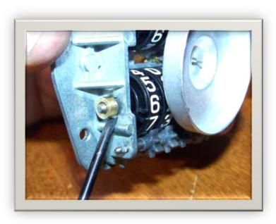
First, go back up a few steps and remove the outside gears.
