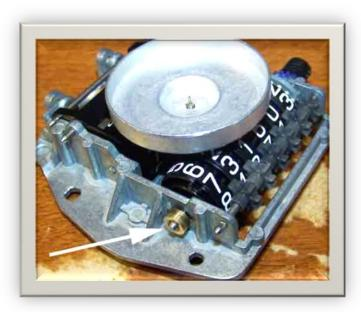
See this **brass collar**? It's pressed onto the shaft (opposite end from the outside gears). This shaft goes through the odometer number wheels and through the two outside gears on the other side. When you try to spin the outside gears (while holding the wide black inside gear steady), **have a look at this collar** to see if the shaft is spinning along with them.
