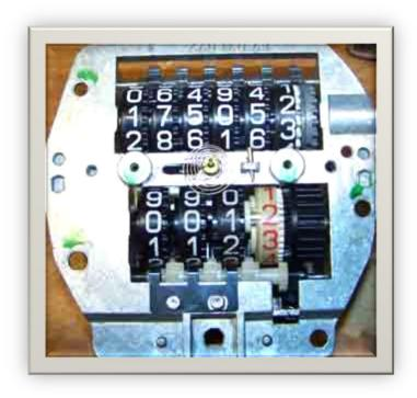
After you re-insert the gray metal gear, push the shaft back through and test the odometer function again before installing the outside gears. Pay attention to the alignment of the top odometer numbers. The first time I re-installed the gray metal gear, I found the far right number wheel was no longer aligned (see photo). This means I allowed that number wheel to slip or the gray metal gear was installed slightly off the mark.
