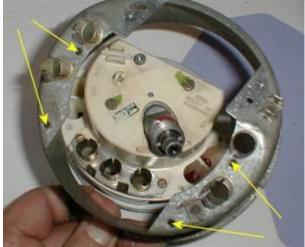
5. From the back of the unit, remove the 2 slotted screws that secure the odometer into the white, plastic assembly and remove the odometer assembly.
