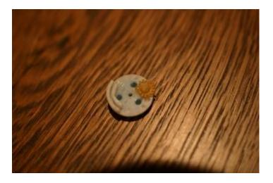
See the broken gear - and its yellow decay - compared to the new gear.
