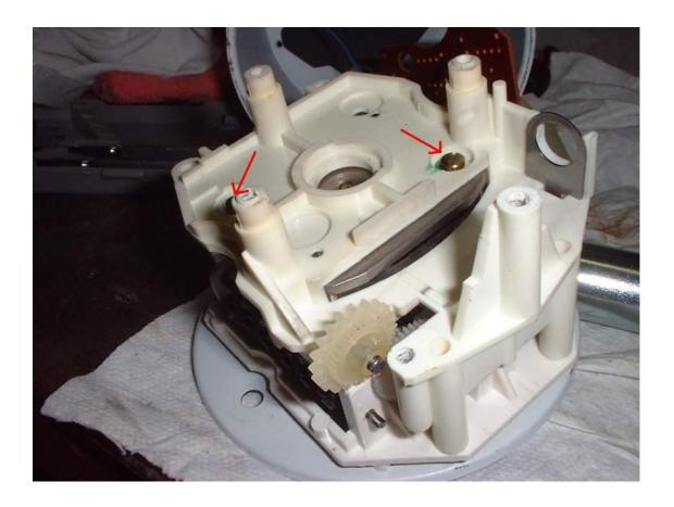
9. You now have access to the axle of the other gear that's in your way. Use a tiny drill bit, needle, or toothpick to push that axle out and you can remove that gear.
