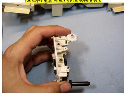
Next, set the black intermediate gear in place and again check for smooth operation. It took me two or three attempts at filing the "knots" off in order to get it perfectly smooth enough to pass this test.
