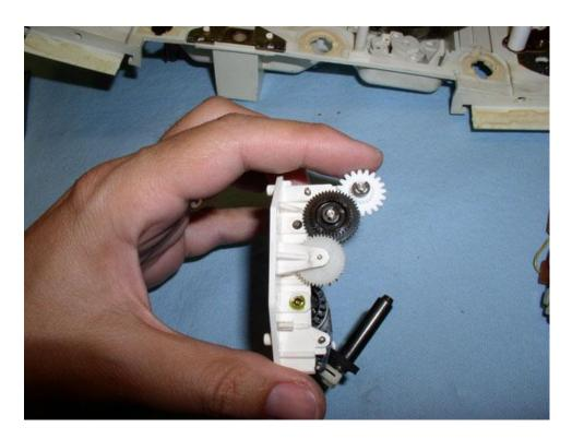
7. You'll also need to remove the drive motor's one screw and pull that out of your way.
