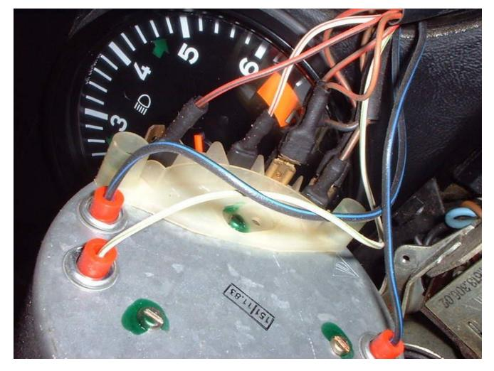
4. Now, for the first fun part: If you're feeling at all tense or agitated, put the **Speedo** on your bench and get a beer or call it a night and return the next day. Removing the bezel and lens is done by many, many small prying motions along the lip of the press-fitting that holds the black bezel that you see from the driver's seat onto the silver aluminum housing that is normally out of sight.
