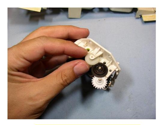
....and insert the drum gear pin as pictured below.
