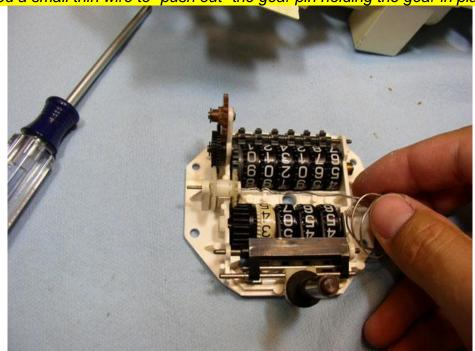
Once the gear pin is partially out, grasp it with some needle nose pliers...
