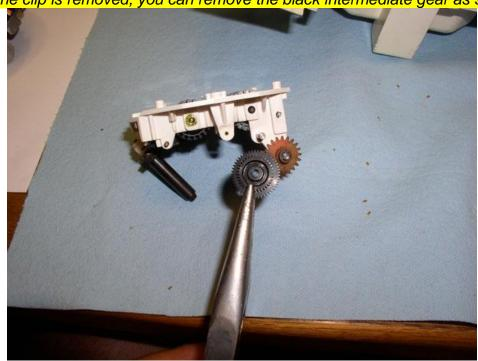
Next, remove the circlip from the first gear wheel in the same manner as the intermediate gear.
