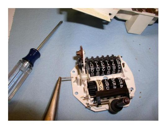
After the pin is removed, you can grasp the drum gear with the needle nose pliers as shown and remove.
