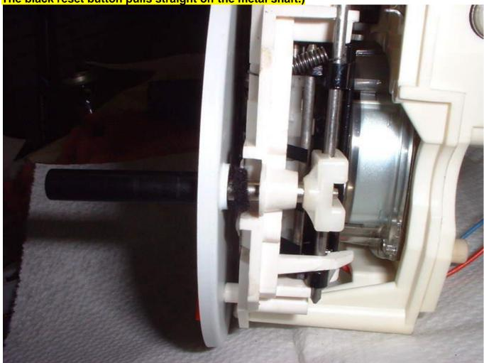
(See below for needle removal instructions. You will have to remove the trip meter reset knob to accomplish this. In the photo above you can see that the reset button attaches to a metal shaft. With one finger gently pull the metal shaft towards the rear of the speedometer. With your other hand unclip the white retainer from the shaft by pivoting the clip sideways. Once you are unclipped remove the reset shaft)
