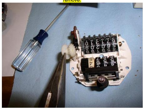
Next, you will need to remove the black intermediate gear. This gear and the first gear are held in place by a very small circlip. I used a small flat blade screwdriver to pry off the clip. Be very careful when prying the clip off as it can fly off and get lost. To prevent loss of the clip, I cupped my hand
