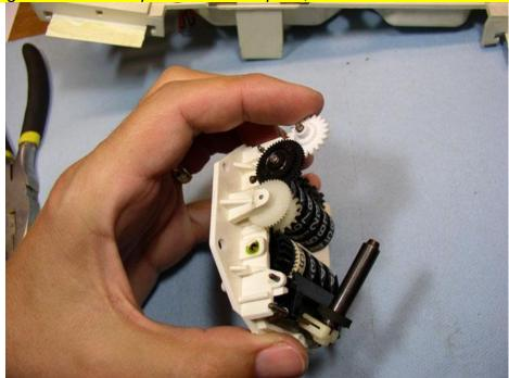
Re-install the small circlips on the intermediate gear and the first gear.
