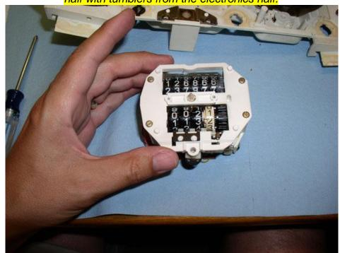
After the screws are removed, carefully separate the two halves by lifting up on the odo tumblers section as shown.
