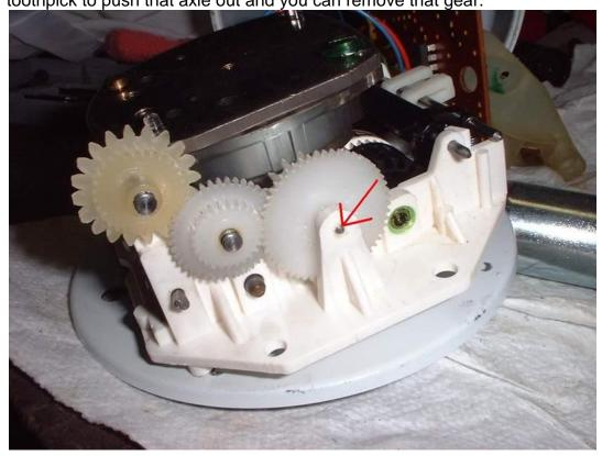
10. They're already removed in the pics, but you also need to remove the gear retainer circlips with a small screwdriver
