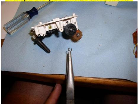
After the clip is removed, you can remove the black intermediate gear as shown.
