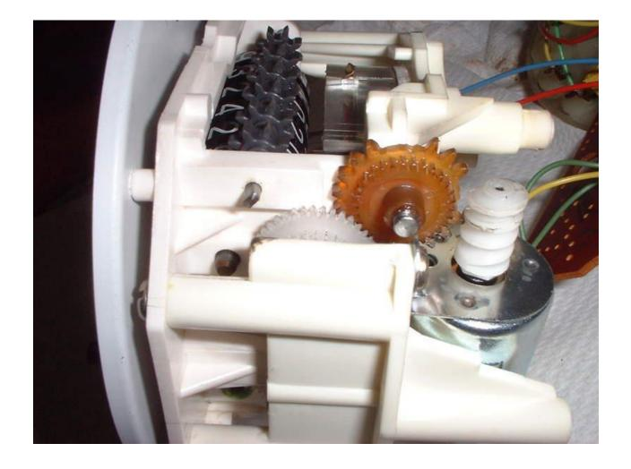
If not, you may not have the same issues as I and so many others before me. I ordered my replacement gear from <a href="www.odometergears.com">www.odometergears.com</a> – it was just under \$30 with shipping for an acetal plastic gear smaller than a quarter and weighing a few grams. But, it beats the \$150 to pay a **Speedo** shop.
