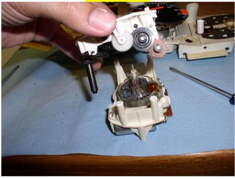
Next you need to remove two gears in order to get at the failed gear. To remove the drum gear, I used a small thin wire to "push out" the gear pin holding the gear in place.
