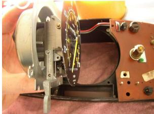
Gently lift the edge of the gauge cluster closest to the Speedo. Lift out the Speedo and pay close attention to the trip meter reset arm, which is why we lifted up the gauge cluster. This makes it much easier to get the Speedo in and out of the cluster without damaging the reset arm.
