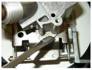
Ahhh we found the problem! The pot metal gear that the screwdriver is pointing to should NOT be turnable without the entire shaft and numbers advancing. This gear in fact does "slip" on the shaft, hence the numbers
