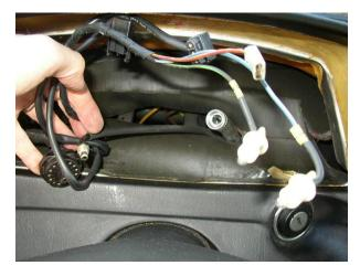
Disconnect the master harness for the gauge cluster. It is usually quite tight so just pull gently straight out, don't rock it side to side. This is the whole harness for the cluster.
