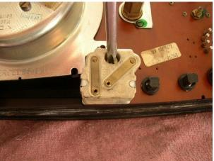
Remove the 2 screws holding the gauge cluster and the dimmer switch. If your dimmer switch does not work, now would be a great time to replace it.
