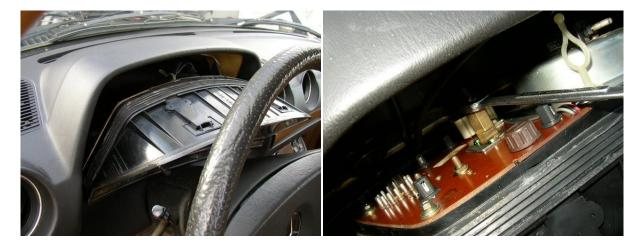
This is why you want some slack on the Speedo cable. The cluster can move forward allowing you to get your hand behind. Remove the oil supply to the gauge with a 10mm wrench.
