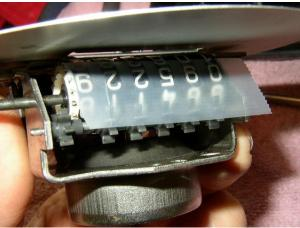
This is by far the hardest part! Putting the geared shaft back into the number set and getting the pot metal gear back into position. It took me about 1 hour to do it. There is very little clearance and the shaft obviously must be out at the point where the gear is slid back in. This causes the other numbers to move and often fall out.
