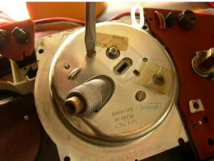
Remove the Speedo electrical box. Then the 2 screws holding the rear of the Speedo.
