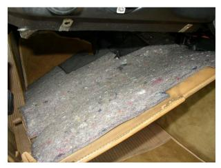
Remove the hush panel under the driver's side dash. There are 3 Phillips screws on the top and 2 plastic Phillips half turn locks, 1 on each lower side.
