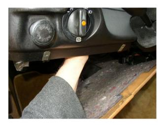
Reach under the dash and gently pull the odometer cable an inch or 2 through the firewall. This will give you a little more room to get your hand behind the dash cluster when you loosen the cluster.
