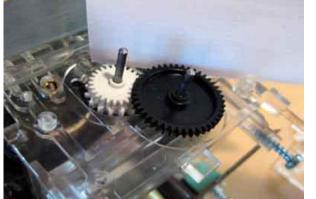
These are the gears that are not replaced in the VDO unit. If you have a MotoMeter unit then only one gear is not replaced.
