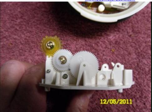
{ODG: The amber colored gear comes in six different tooth counts. You have to count the teeth on your old gear before ordering. 20x21, 20x22, 20x23, 20x29, 20x30 or 20x32 these can be ordered directly through Odometer Gears LTD:
