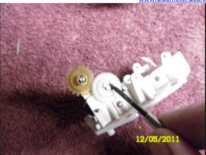
{ODG: Remove the c-clip that secures this gear and the amber gear. Be careful and place a cloth over the unit when removing so that you do not loss the clips. Clean the shaft that the amber gear rides on as any residue from the old waxy gear can cause the unit to either work erratically or not at all. It is also recommended to inspect the hour numbers as well as the main housing and works for any flakes or debris of the old gear and remove. }
