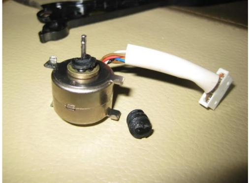
Once the motor is removed you will see the worm gear attached to the bottom side of the motor. Remove the old worm gear by pulling it off with your fingers or a flat blade screw driver. Install the new worm gear using channel lock pliers or a bench vise leaving the thickness of two business cards between the motor and the gear.
