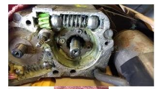
**!!!NOTE:** If you remove the large gear there is a plastic thrust washer that is generally stuck to the bottom of the gear with grease. Remove the washer and align with the four screw heads inside of the housing. Reinstall the gear. If you do not have the washer aligned properly you will not be able to secure the cover as it will not sit flush!!!
