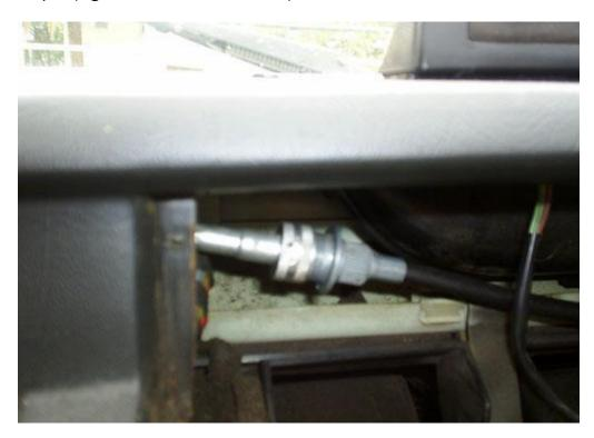
Unscrew the speedometer cable. The connection is underneath the air vent in the centre of the dash. Simply unscrew the cables and pull apart.
