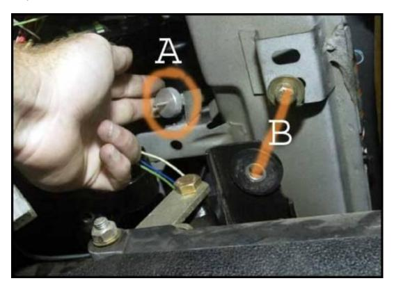
Unscrew the knob (A) and remove it from the track it is sitting in. This cable holds the cluster in tight to the dash. It sits in a metal track mounted to the frame of the car.
