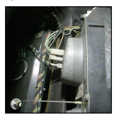
There are a few wires you will have to pull to disconnect the tach and other gauges. They should stay in the correct location after you disconnect them but make a note for re-installment.
