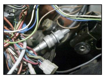
Unscrew the speedometer cable. On automatics or manual vehicles, the cable will always have a link under the rat's nest of wires to the left of the steering column. Simply unscrew the cables and pull apart.
