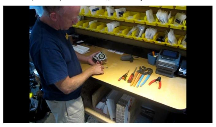
Using a small screwdriver at one corner, wedge the screwdriver between the housing and the metal plate.
