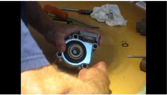
Insert a long screwdriver from the motor side under the gear assembly and while prying up with the screwdriver with one hand gently twist the gear assembly with the other hand. This helps to keep from damaging the internal seal as this is not available without purchasing a new assembly from BMW.
