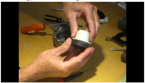
Next you want to use brake cleaner to remove any residue or debris from the gear housing. Apply a layer of high temperature or marine axle gear to the new gear. Reinstall in the reverse order.
