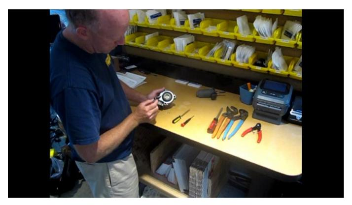
Tip over assembly and remove the washer, you will be reusing this washer do not lose.
