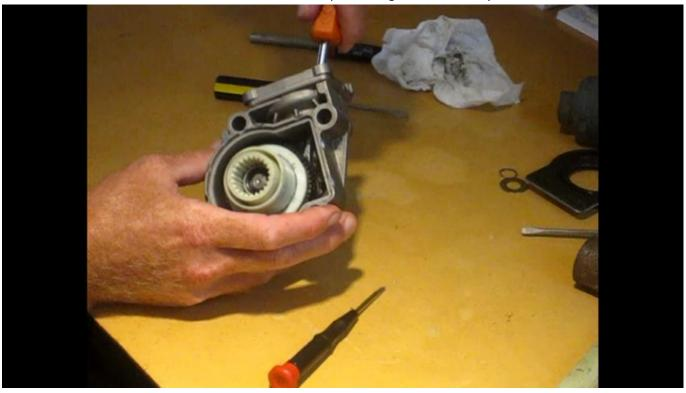
Grasp the white gear with one hand and the black gear with the other, wiggle the two parts apart.
