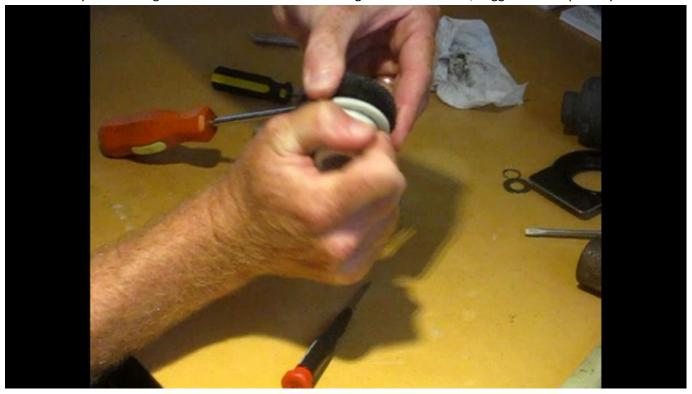
The material we use to reproduce this gear is a high temperature nylon material with carbon fiber reinforcement.
