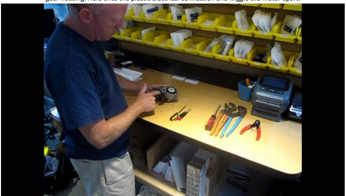
Motor and electrical connection removed as one piece. This ensures that the motor contacts do not spring out making reinstallation harder.
