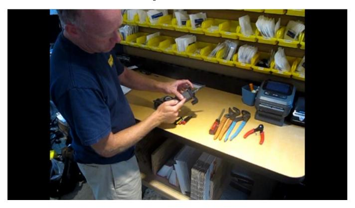
Using several size small screwdrivers, wedge behind the c clip inside of the white gear, you will be reusing this clip so do not lose.
