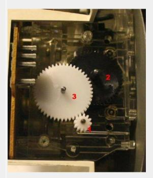
Go ahead and reinstall the clear plastic cover now, making sure the two shafts marked in the picture below mate up with their respective holes in the cover. Replace the two screws that hold it in on. Voila! You now have a working odometer!
