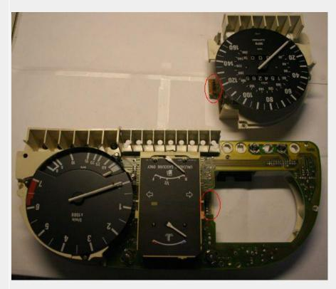
Looking at the speedo section (now separated), you should be able to locate the odometer gears easily behind a clear plastic cover. Remove the two highlighted screws to access them (shown below). I've numbered the 3 gears which you should have received in your package, these are the ones you'll be replacing.
