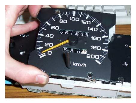
On the side of the Speedo there is a gold motor with two black Phillips-head screws holding it on. Remove these screws and pull the board aside:
