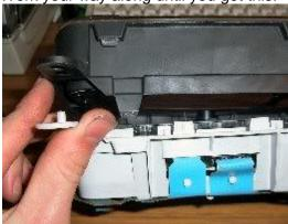
And then just lift it off. You only need to undo the bottom clips then basically just pull it off the cluster:
