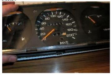
Now lift the Speedo out of the cluster housing and put the housing aside for now:
