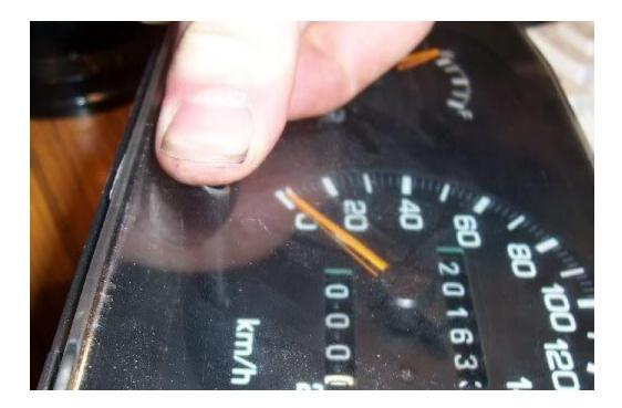
Now plug it back in and take it for a test drive before you put all the covers back on the dash. Just make sure you plug the hazard switch in or your indicators won't work... and don't get too distracted by the odometer moving
