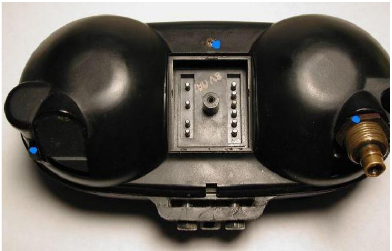
Photo 1. Remove these three screws and Speedo cable nut.
