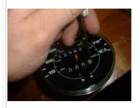
The internal workings of the speedometer with the face removed. Before installing the outer gear use a center punch to gentle tap the odometer shaft out. You only want to remove this shaft just far enough to remove the lead gear. Install the new lead gear in place and use a large pair of channel lock pliers to gently press the odometer shaft through the new lead gear. You do not want to squeeze this together to tightly as the assembly must still be able to spin freely. Now install the outer gear
