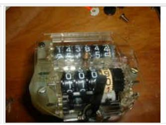
Reinstall the odometer face and just tighten the screws until they touch the face.
