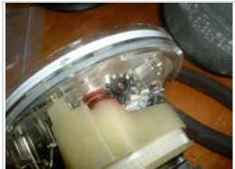
If this gear is bad, use a flat tip screwdriver under to gear to pry off. Press on the new gear with your fingers or a large pair of channel lock pliers. Just inside the speedometer clear plastic housing is located the lead gear that must fit tightly on the shaft in order for the odometer to work correctly. If this spins on the shaft it must be replaced as well.
