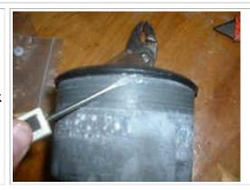
Then use a larger screwdriver to work around again. Eventually the bezel will slide off easily.
