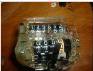
Reinstall the odometer face and just tighten the screws until the screws just touch the face plate. Excessive tightening will damage the face of the screw.
