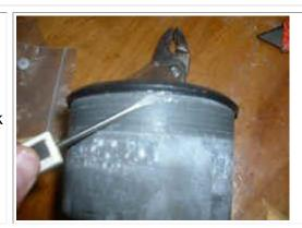
Then use a larger screwdriver to work around again. Eventually the bezel will slide off easily.
