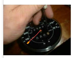
From the backside of the speedometer there is an opening that you are going to put a small mechanics standard screwdriver through. Place the tip of the screwdriver between the metal canister and the internal speed cup. Then lightly twist the screwdriver to lock the speed cup into place. *Do NOT* put a lot of torque on the screwdriver as it is not needed and could damage the speed cup.
