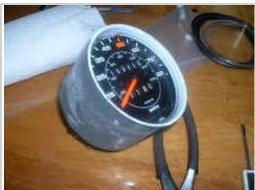
The two screws in the back of the speedometer are removed.
