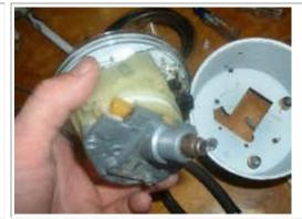
The small black gear is the one that either cracks or does not hold tightly to the odometer shaft any longer. Need to count the teeth in order to order the correct replacement gear. It is always best to remove your speedometer and count the teeth of your old gear first. Most US Spec vehicles are 17 and most European Spec is 11.
