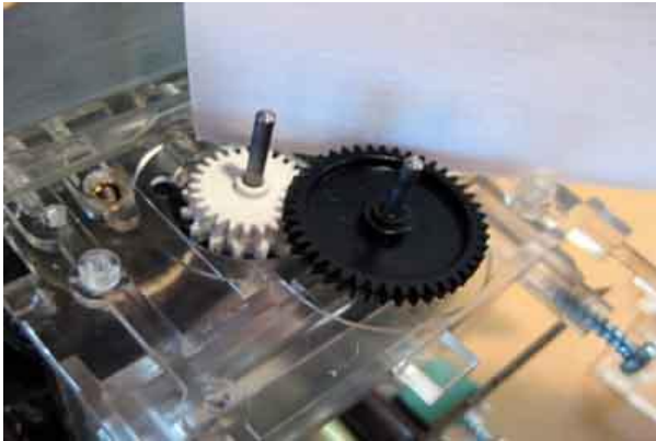
These are the gears that are not replaced in the VDO unit. If you have a MotoMeter unit then only one gear is not replaced.
