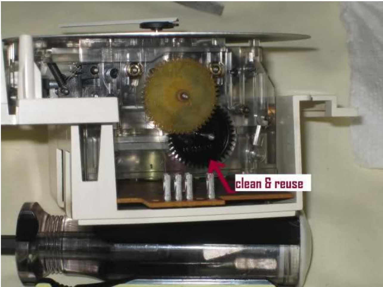
The following photo shows the new gears installed, just before replacing the clear plastic cover.
